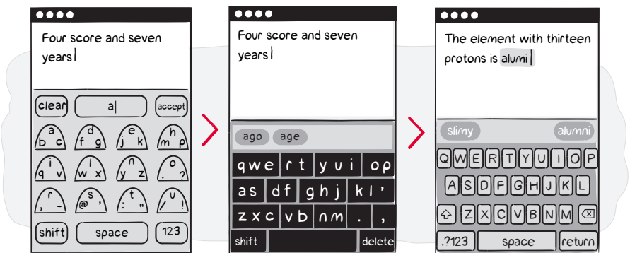
FIGURE 8.3 Incremental Prototypes of the Apple iPhone Keyboard
